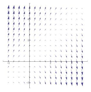
For any Differential equation of the form y' = F(x, y) we can make a **direction field** by drawing an arrow with slope F(x, y) at many points in the plane. The more points we include, the better the picture we get of the behavior of the solutions.
